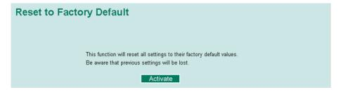
This function provides users with a quick way of restoring the Moxa DSL Ethernet extender's configuration to factory defaults. The function is available in the serial, Telnet, and web consoles.
