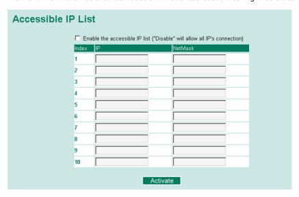
You may add or remove IP addresses to limit access to the Moxa DSL Ethernet extender. When the accessible IP list is enabled, only addresses on the list will be allowed access to the Moxa DSL Ethernet extender. Each IP address and netmask entry can be tailored for different situations:
