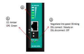
**NOTE** If the DSL link can't be finalized within 7 minutes, please check line conditions and configurations: e.g. distance, speed setting, environmental noises, etc.
