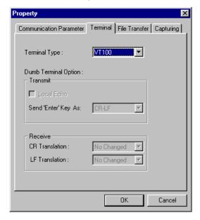
5. In the terminal window, the Moxa DSL Ethernet extender will prompt you to select a terminal type. Enter 1 to select ansi/vt100 and then press Enter.
