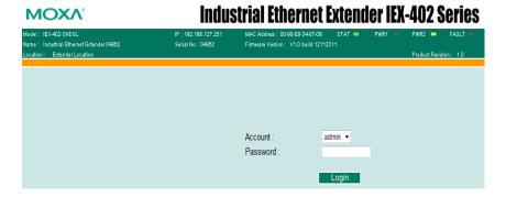
**NOTE** By default, no password is assigned to the Moxa DSL Ethernet extender's web, serial, and Telnet consoles.
