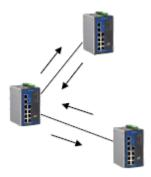
From the DSL Ethernet extender's web interface, you can enable or disable LLDP, and set the LLDP transmit interval. In addition, you can view each DSL Ethernet extender's neighbor-list, which is reported by its network neighbors. Most importantly, enabling the LLDP function allows Moxa's MXview to automatically display the network's topology and system setup details, such as VLAN and Trunking, for the entire network.
