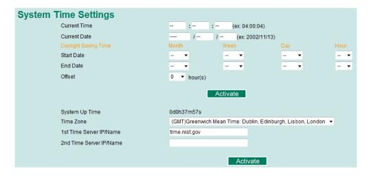
The Moxa DSL Ethernet extender has a time calibration function based on information from an NTP server or user specified time and date. Functions such as automatic warning emails can therefore include time and date stamp.
