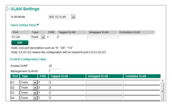
When VLAN Mode is set to 802.1Q VLAN, the configuration options will be divided into the **Quick Setting Panel** and **VLAN ID Configuration Table**. The Quick Setting Panel is generally used to configure VLAN settings for groups of ports, with the settings pushed down to the VLAN ID Configuration Panel when the user clicks the Add button. The VLAN ID Configuration Table can be used to configure the settings for individual ports.
