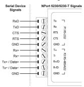
NOTE The NPort 5232/5232I/5232-T/5232I-T have 2 RS-422/485 ports. The pin assignments are the same as the NPort 5230/5230-T's port 2. Refer to the "NPort 5200 Series User's Manual" for more details.
