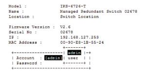
7. The **Main Menu** of the Moxa switch's serial console should appear. (In PComm Terminal Emulator, you can adjust the font by selecting **Font...** from the **Edit** menu.)
