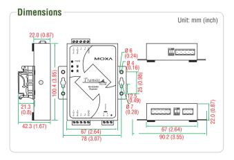
Input Voltage: 12 to 48 VDC **Power Consumption:** TCC-120: 65 mA @ 12 V TCC-120I: 180 mA @ 12 V
