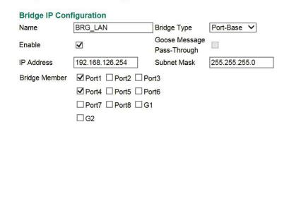
First, select **Port-Base** in Bridge Type. Then input a name for the Bridge interface and assign an IP address/Subnet Mask for the interface. In order to enable this feature, checkmark the Enable checkbox. Finally, please select the port that will be set as the bridge port and check Apply.
