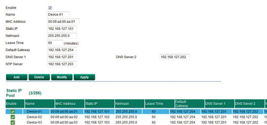
In the above example, a device named "Device-01" was added to the Static DHCP list, with a static IP address set to 192.168.127.101 and MAC address set to 00:09:ad:00:aa:01. When a device with a MAC address of 00:09:ad:00:aa:01 is connected to the Industrial Secure Router, the Industrial Secure Router will offer the IP address 192.168.127.101 to this device.
