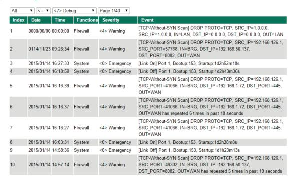
By default, all event logs will be displayed in the table. You can filter three types of event logs, **System**, **VPN**, and **Firewall**, combined with **severity level**.
