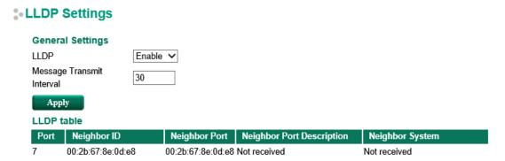
The router's web interface can be used to enable or disable LLDP, and to set the LLDP **Message Transmit Interval**. Users can view each switch's neighbor-list, which is reported by its network neighbors.
