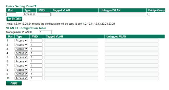
Input the port numbers in the Port column, and set the Port Type, Tagged VLAN ID, and untagged VLAN ID. Next, click the **Set to Table** button to create the VLAN ID configuration table.
