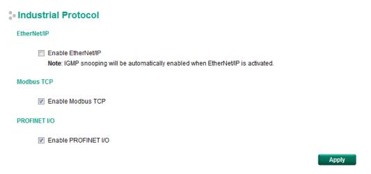
The default PROFINET I/O setting of EDS E series is disabled. To enable the PROFINET I/O support, check the **Enable PROFINET I/O** and click **Apply**.
