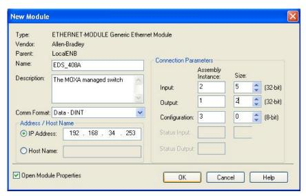
5. After finishing configuration, the new Ethernet module representing the Moxa Ethernet switch will appear under the **I/O Configuration** list in the controller organizer window.
