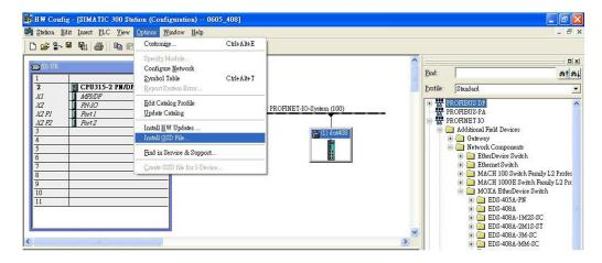
5. You will find the new MOXA switch under PROFINET IO > Additional Field Devices > Network Components > MOXA EtherDevice Switch.
