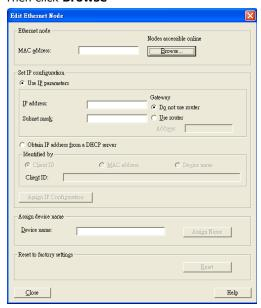
Click **Start** to search devices. Use STEP 7 through PROFINET DCP to discover devices in networks. Find PLC/switch IP addresses, MAC addresses, and device names here.
