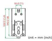
The DIN-rail kit is attached to the back panel of the OnCell G3470A-LTE series. Mount the OnCell G3470A-LTE series on corrosion-free mounting rails that meet the EN 60715 standard.
