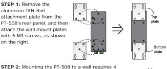
**STEP 2:** Mounting the PT-508 to a wall requires 4 screws. Use the PT-508, with wall mount plates attached, as a guide to mark the correct locations for the 4 screws. The heads of the screws should be less than 6.0 mm in diameter, and the shafts should be less than 3.5 mm in diameter, as shown on the right.
