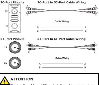
This is a Class 1 Laser/LED product. To avoid causing serious damage to your eyes, do not stare directly into the Laser Beam.
